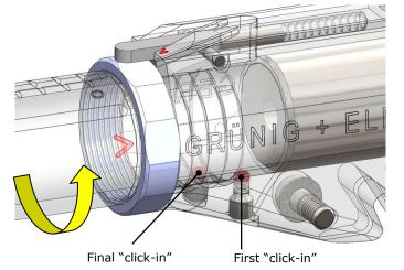
Tighten the left-threaded lock nut **counter-clockwise** using the special tool
