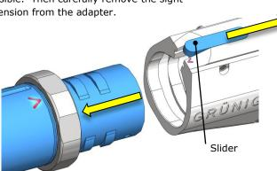
Push the slider back with your thumb as far as possible. Rotate extension tube counterclockwise until the two marker arrows align. You should feel the "click-in" of the detent ball.
