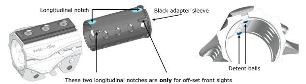
**Check:** When the adapter sleeve is installed correctly, the two position notches of the sight base tunnel and the adapter sleeve will align perfectly.
