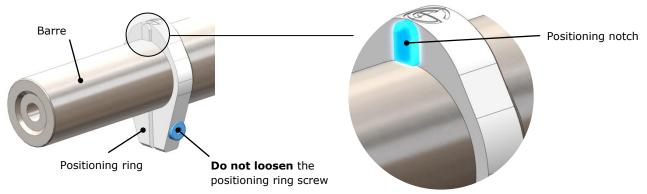
The lock screws of the adapter must be loosened first. You can then slide the sight extension onto the barrel. Join the positioning groove of the adapter with the position notch of the positioning ring. Then tighten the lock screws of the adapter.
