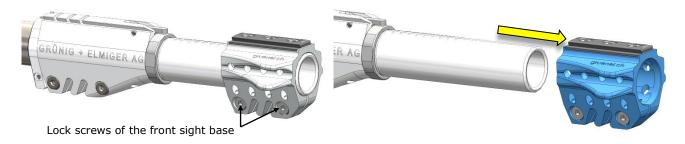
To attach the front sight base directly to the barrel, you have to insert the black adapter sleeve into the front sight base. The adapter sleeve bridges the gap from the barrel diameter (20mm) to the front sight diameter (23mm). Please make sure that the two detent balls lock into the two indentations of the adapter sleve.
