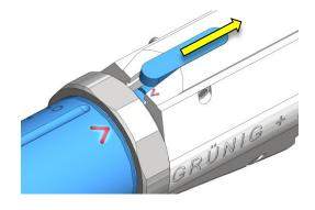
Rotate the extension tube clockwise until you feel the detent ball "click-in" at 60°.
