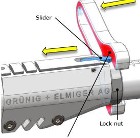
Push slider back with the special key so that it is flush with the lock nut.
